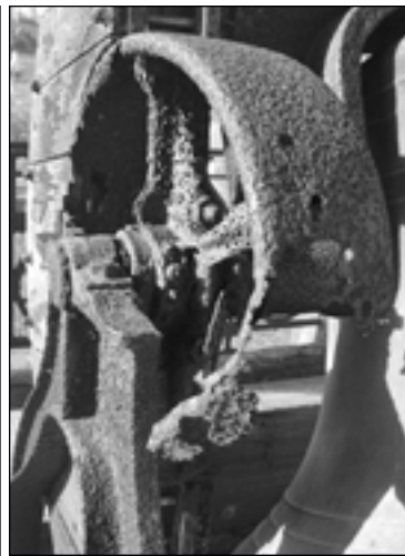
BELOW: The Rogers School Bell was cast in 1885. ABOVE: Two angles of the corroded cradle. The bell will be removed on Saturday at 10 a.m. Committee members hope to have it re-installed after getting the cradle rebuilt. Submitted photos.
